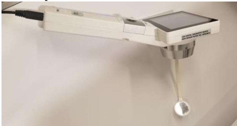
FIGURE 2 Horus Scope Camera with Dental Lens Attachment
